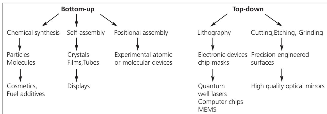
Figure 4.2 The generic processes that are involved in the production of nanoparticles
