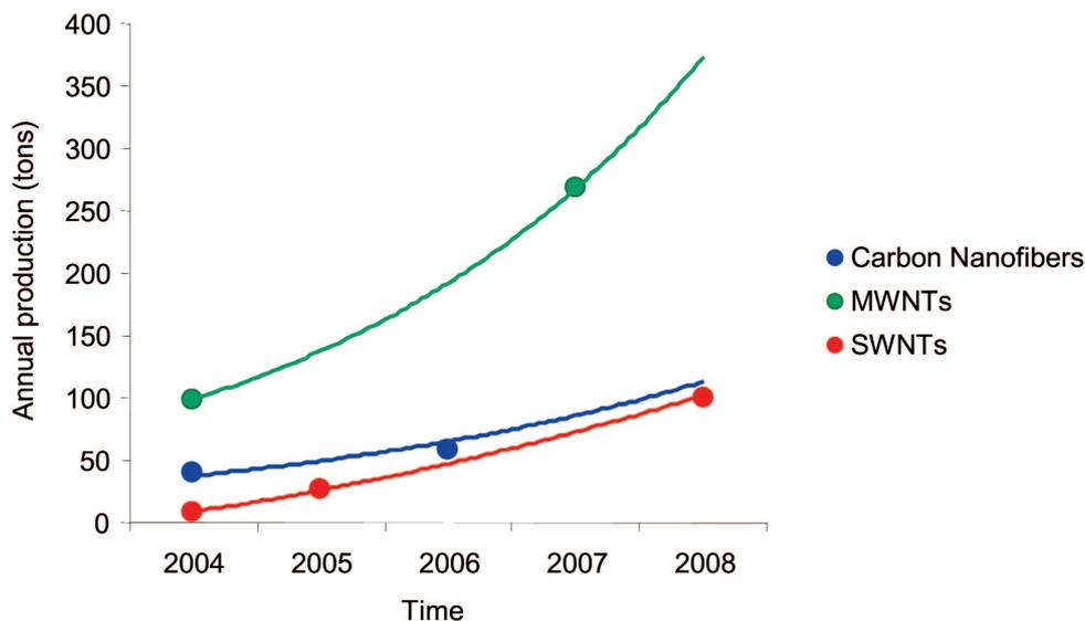
currently produced). This is an area of intense research. Current production capacity for CNTs is estimated to be around 100 tonnes per annum (Cientifica 2004); the actual production output remains commercially confidential, but is expected to be lower. Most of the capacity is estimated to be multi-walled tubes, with single-wall tubes accounting for about 9 tonnes of capacity. Estimated future global production of nanotubes is outlined in Figure 4.3.
